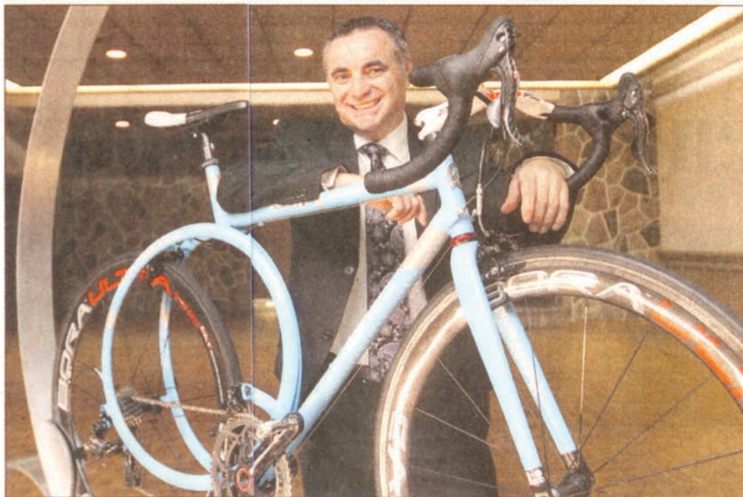
Windsor entrepreneur Lou Tortola unveils his innovative bicycle design at the Caboto Club on Saturday. The RoundTail bicycle design helps to reduce stress on the rider's spine by absorbing the impact through the two adjacent circles.
