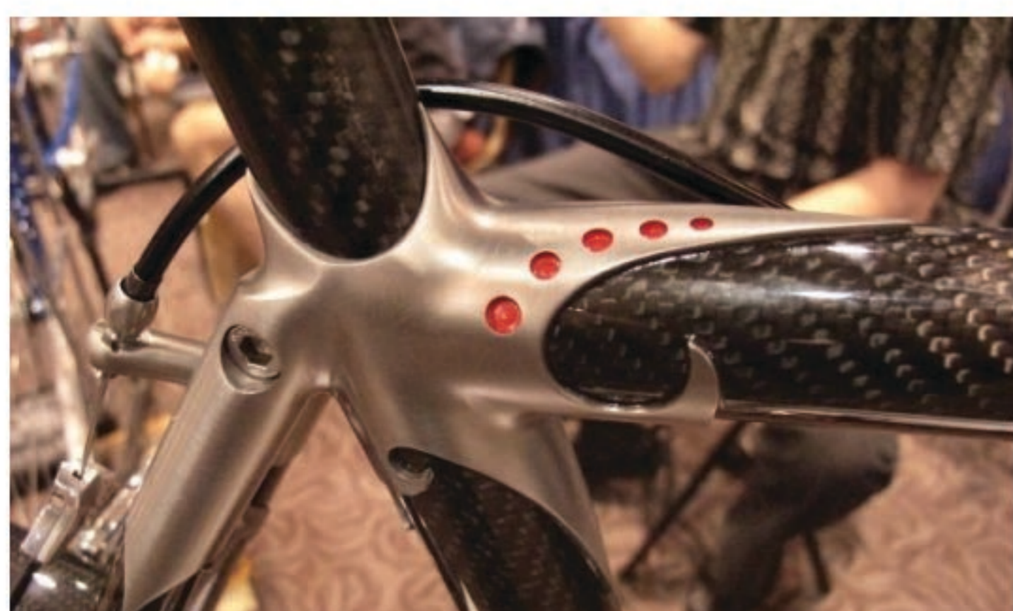
Last year Bruce Gordon showed off a carbon bike with ti lugs he built with Mike Lopez. This is #2 of 2. I dare anyone to try to find prettier work that has been performed in titanium. The tapered design kills me.
