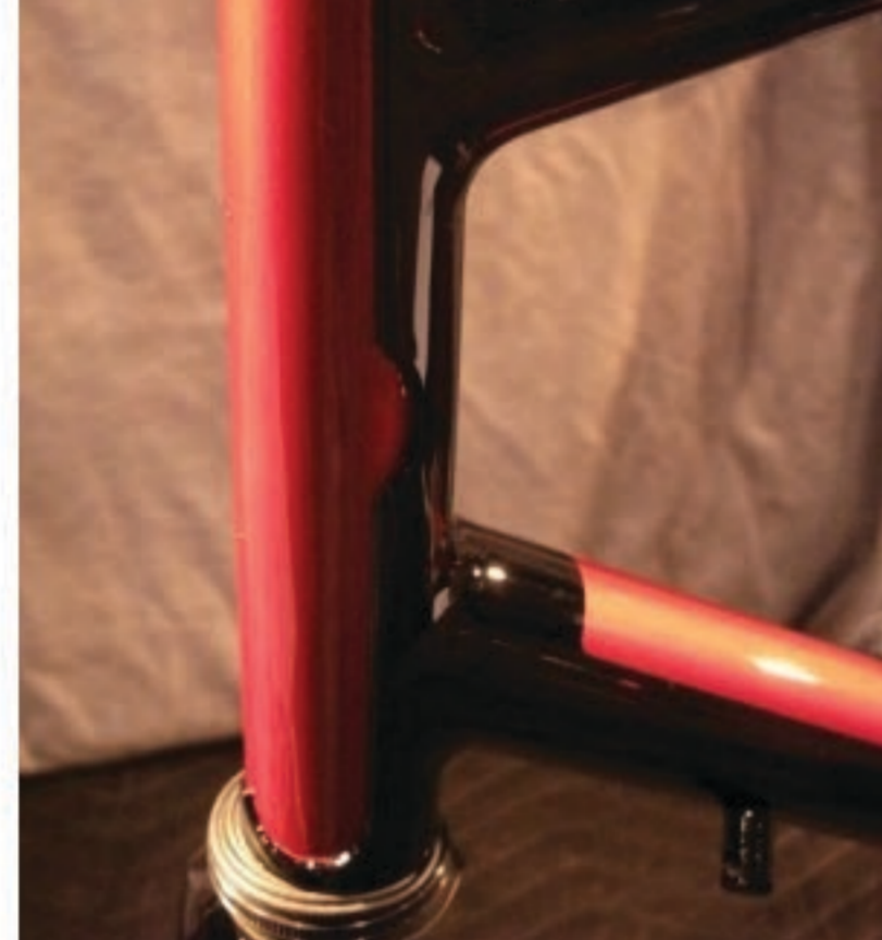
Eric Estlund of Winter Bicycles is fond of bi-laminate work. This head-tube cutout was gorgeous. The bi-laminate approach gives him the opportunity to show off his fillet brazing as well as his ability to cut lugs.
