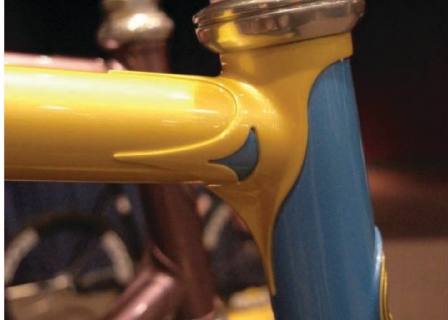
Brent Steelman is probably best known for his welding, but his lug work is outstanding, as seen in these arrow point lugs. The windows he cut in each of the lugs reflected the shapes of the points.
