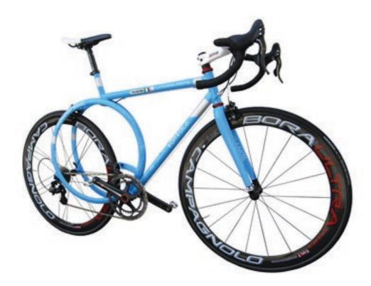
A Canadian inventor has unveiled a new bicycle frame design that he claims is dramatically more comfortable than a traditional double diamond layout while retaining the same lateral stiffness and pedaling efficiency.
