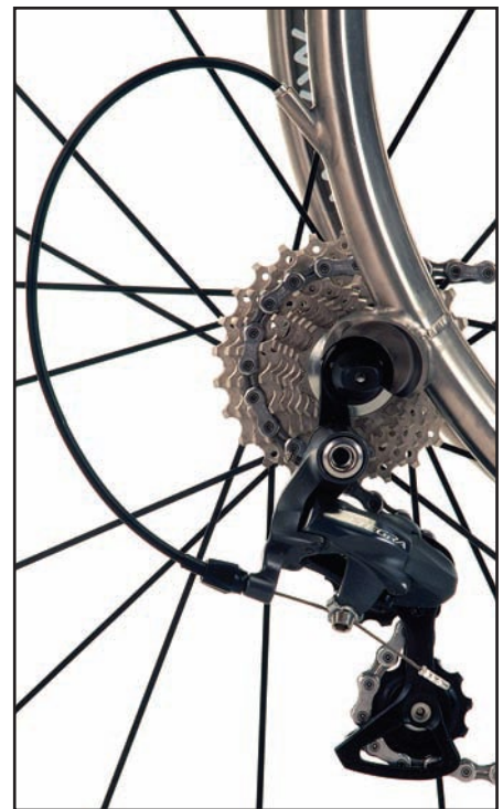
Stout dropouts and internal rear derailleur cable routing were nice touches.
