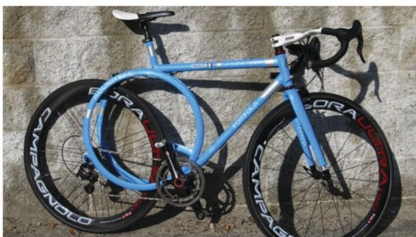
The Tortola RoundTail bicycle replaces the frame's traditional rear triangle with two shock-absorbing joined rings (All photos courtesy Lou Tortola)
